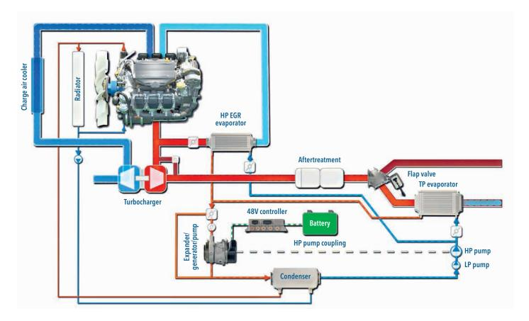
manufacturer Mahle has approached the problem slightly differently. While its WHR system also works on the Rankine cycle, almost all of it is packaged into a single 55cm-wide box designed for easy installation into a variety of vehicles.
